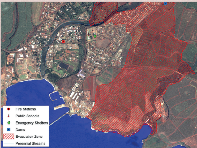
Maps of potential downstream flooding resulting from a dam break scenario were used by officials in Hawaii to delineate evacuation zones.
