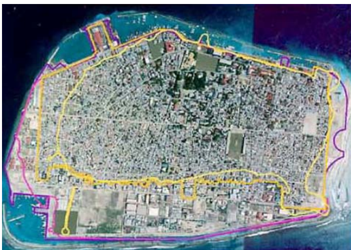
PDC's DPMA time/space analysis showing the "growth" of Male Island, Maldives, over several decades. Coral is mined from nearby atolls, processed, and used as landfill to increase the size of the island. The yellow outline shows the original size of the island.
