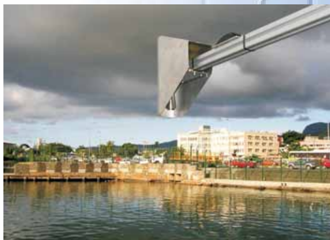
GLOSS sea level stations employ a number of instruments to measure sea level, including down-looking radars to measure sea level. Port Louis, Mauritius. Photo courtesy of University of Hawaii Sea Level Center.
