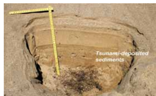
Sediment layers deposited from successive waves of 26 December 2004 Indian Ocean tsunami, as observed in Banda Aceh, Indonesia. Photo courtesy of Yuichi Nishimura, Hokkaido University.
