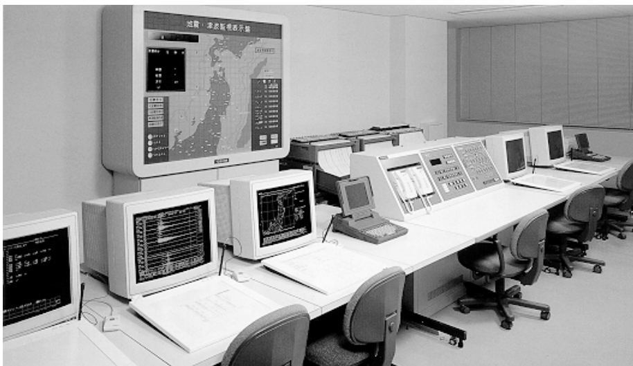
Operations counter for one of six tsunami warning centers in Japan. Seismic signals are continuously monitored, and earthquakes detected and processed with an automatic Earthquake and Tsunami Observation System.
